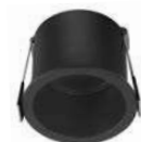
HAP - 9174152 Sandy Black Aluminium LED GU10 1x10 Watt IP20 220-240 Volt Bulb Excluded D: 6.8 H: 5 cm Cut Out: 6.2 cm
