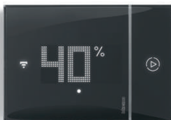
Display the set room temperature and humidity
